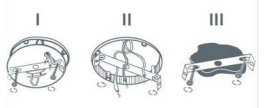
3. Connect the wires to the ceiling lamp:
